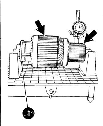
Turning down commutator
